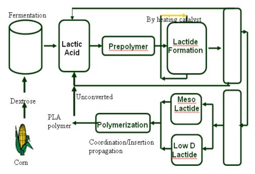
The lactic acid obtained from fermentation of plant substances is used as a feed to synthesize PLA. Then, a continuous condensation reaction of aqueous lactic acid is carried out in order to provide the PLA prepolymer having a low molecular weight.
